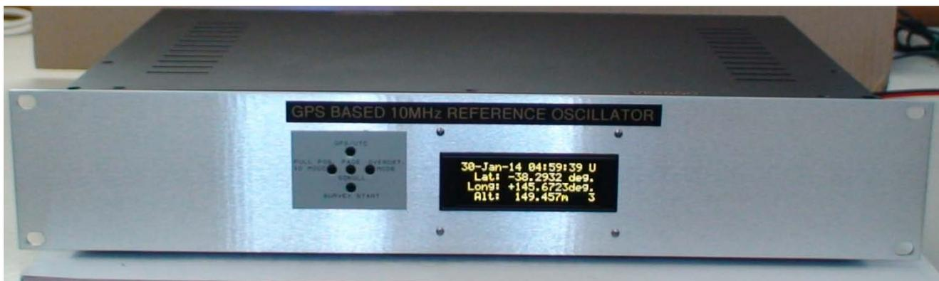
**A display and command module for the Trimble Thunderbolt GPS with 10MHz reference oscillator.**
